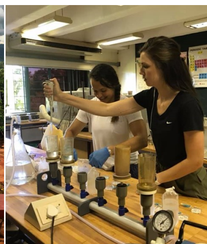
Membrane filtration is used to evaluate water quality samples taken from the field.
