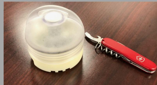
Figure 1. A prototype electrolytic water purifier. The device floats in a water storage container and has silver-wire electrodes on the bottom that disinfect the water.
